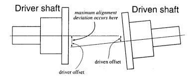
Misalignment exists when the centre lines of two adjacent machines deviate from each other. Alignment related problems include soft foot, pipe strain, inadequate bases etc.
