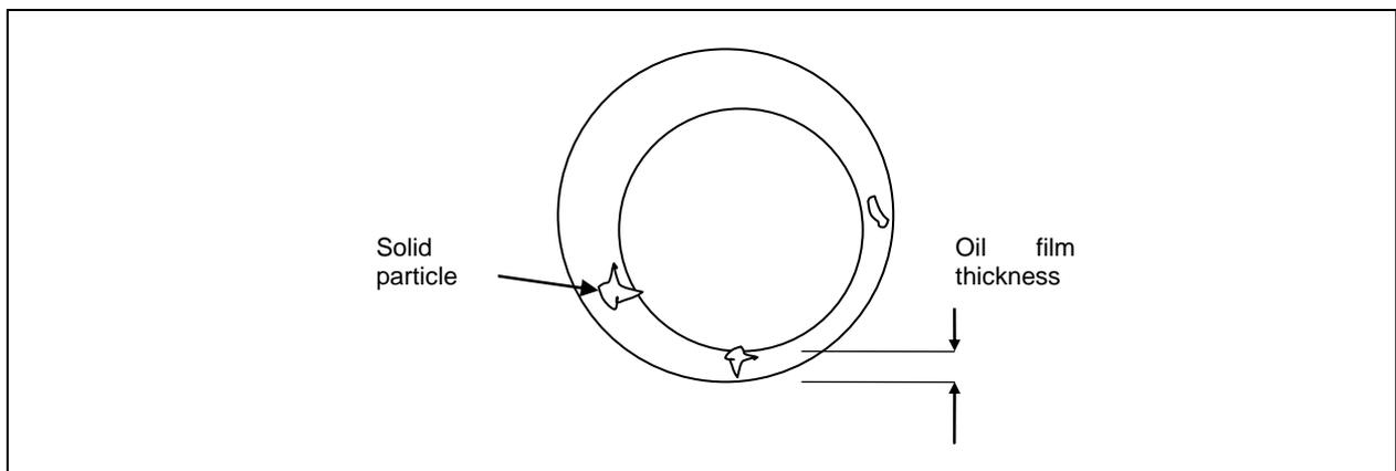
Figure No. 1 Solid Particles in Bearing Oil Film
